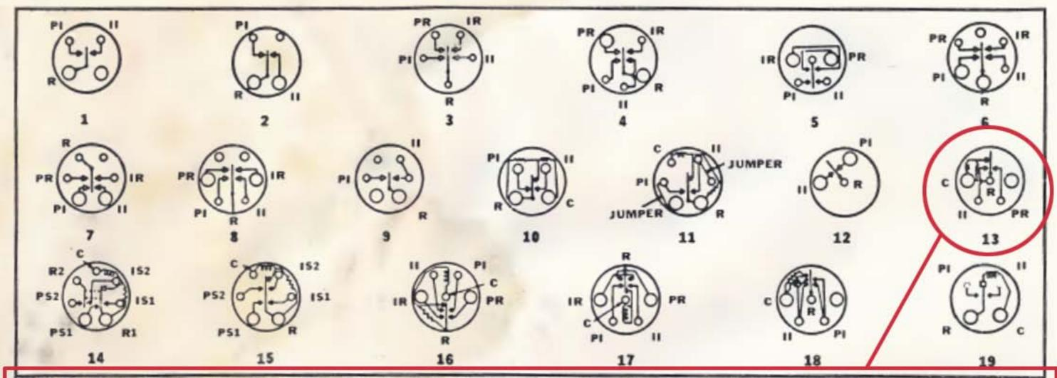
BASE DIAGRAMS: C = Coil; II = Inertia Interrupter; IR = Inertia Rectifier; IS = Inertia Spring; PI = Pull Interrupter; PR = Pull Rectifier; PS = Pull Spring; R = Reed.
