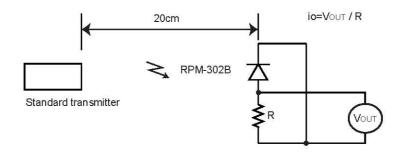
Fig.2 Measurement of standard transmitter proofreading
