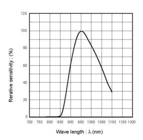
Fig.7 Optical bandwidth of the photo-diode encapsulation
