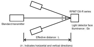
Fig.3 Measurement condition for effective distance
