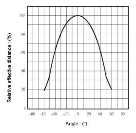
Fig.8 Direction characteristic (Horizontal direction)
