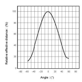
Fig.9 Direction characteristic (Vertical direction)
