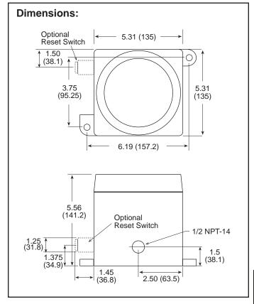
Counter Catalog Number (Use #1 or Clip Mount) 529K.2 MK18.10 24VDC 25CPS KAT-SP
