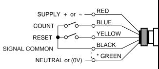
\* Jumper Black to Green for voltages less than 48V DC or AC
