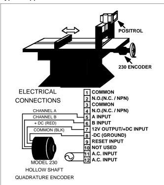
The POSITROL position monitor can be used in many position applications. When two units are used, both X and Y axes positions can be monitored. The application below involves monitoring of the X axis only.
