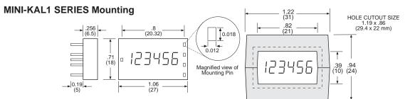
MINI-KAL1 SERIES with KALPM1 panel adaptor clips into panel .050 to .125 thick
