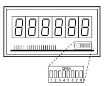
OFF Reset to zero **SW 1** ON Reset to preset
