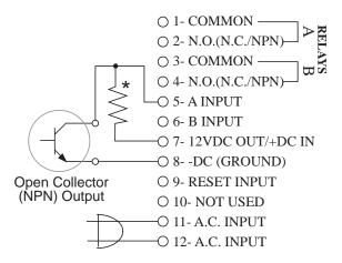
\* Pull-up resistor required for open collector (NPN) outputs.
